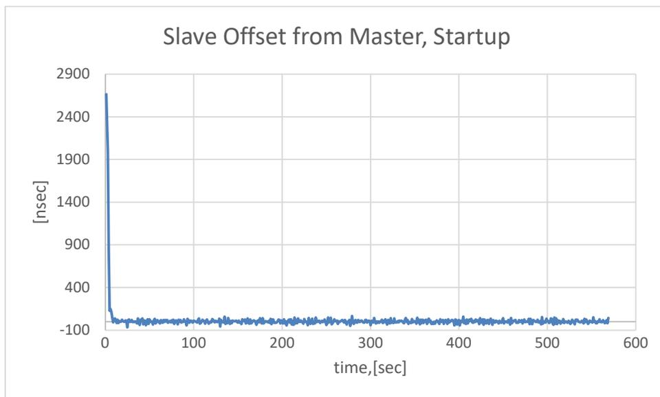
**Figure 3-3. Slave Offset from Master, in Startup State**
